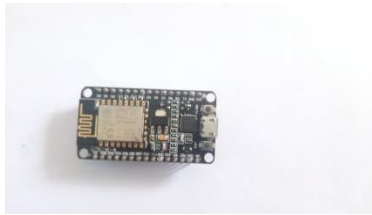
Gambar 1 Board NodeMCU ESP8266
