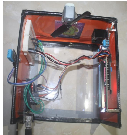
Gambar 7. Perancangan Arduino Uno R3, Breadboard, LCD, Sensor DHT11, LED, Resistor, Driver Motor DC dan Motor DC
