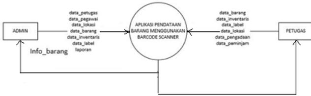
Gambar 2. Diagram DFD level 0
